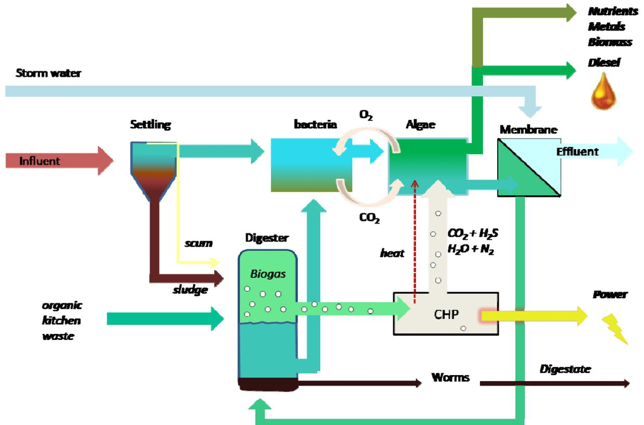
The inflows are: 1.influent consisting of combined grey and black water, 2. The storm water which can be separated from the sewer and 3. organic kitchen waste which is perfect fermenting material.
